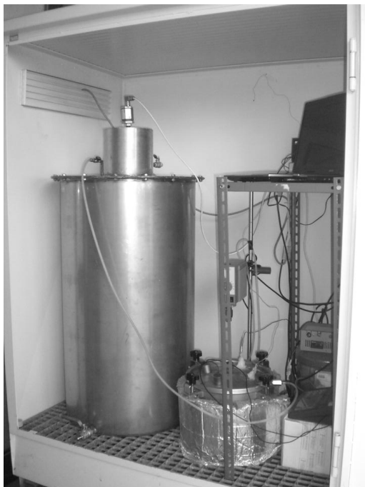
Figure 1: Anaerobic digestion pilot plan
