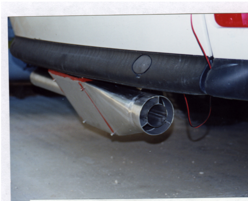
Figure 6: Active Noise Control Muffler
