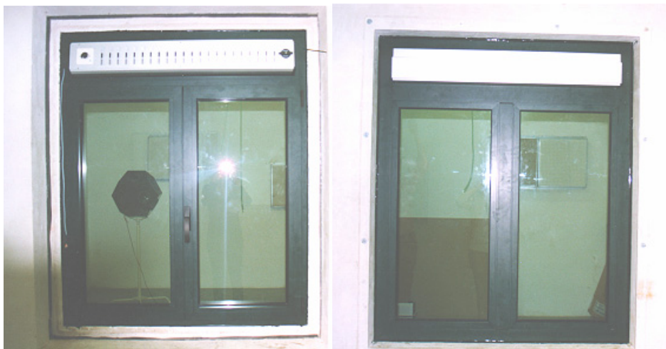
Figure 1: High Sound Insulation Windows
