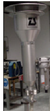
Figure 10. Sampling head for PM10 fraction.
