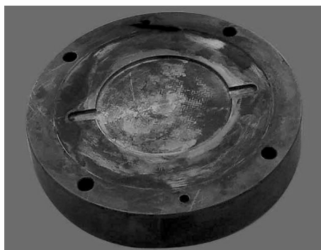
Fig. 9 Picture of the bottom steel plate of the reactor after its disassembly
