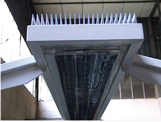
FIGURE 4: Detail of the PV panel and the finned surface.
