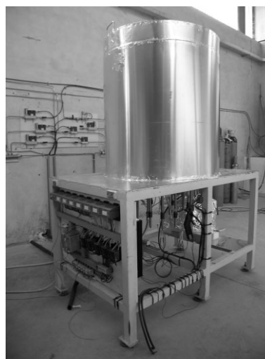
Fig. 11 Picture of the 1 kW final configuration SSMCFC.
