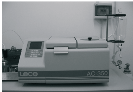
Figura 4: Calorimetro AC-350 LECO (PCS)
