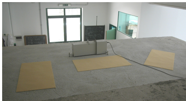
Figure 1. Tapping machine on the floor and positions of the samples.
