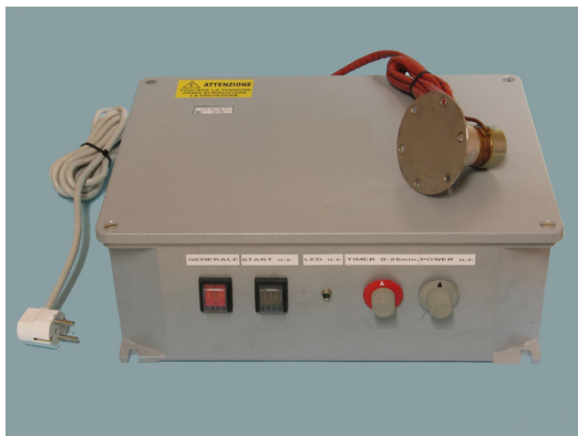
Fig.2. Ultrasonic generator and piezoelectric transducer.
