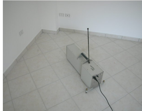
Figure 6: Brick-concrete floor Tapping machine on the floor
