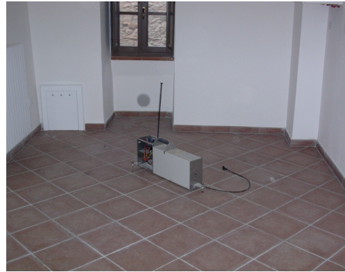
Figure 2: Steel beam floor with sheet Tapping machine on the floor
