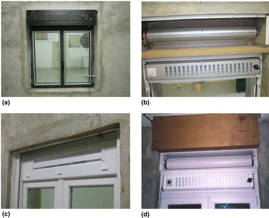
Fig. 4. HSIWV with rolling shutter boxes: (a) sample no. 1; (b) sample no. 2; (c) sample no. 3; (d) sample no. 4.
