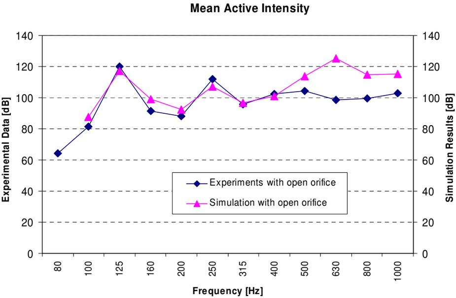
Figure 7: Average sound intensity level recorded and calculated on the planar surface above the AIM (see Figure 2, right), at 2000 camshaft rpm (measurement performed with a 12 mm microphone spacer).
