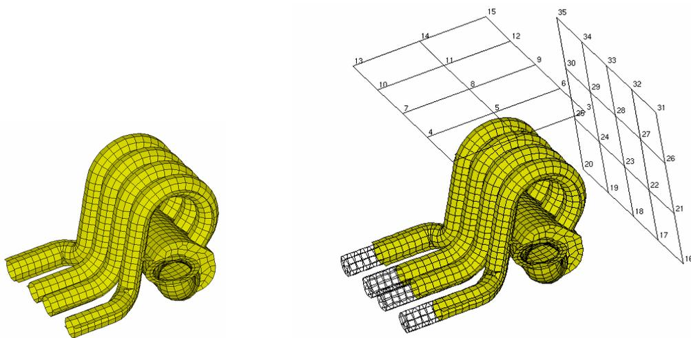
*Figure 2: Simplified shell-element mesh of the AIM used for coupled analysis. On the left, FEM structural model; on the right, superimposed wire-frame BEM acoustic model and field points chosen for post-processing of the results.*
