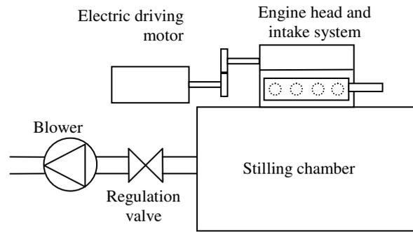
Figure 4: Picture of the dynamic flow test bench, on the left, and schematic of its layout, on the right.
