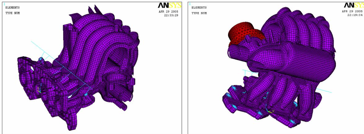
Figure 1: The fully-detailed 2D element mesh of the AIM under test. On the left, AIM without orifice flange mass; on the right, with flange mass.
