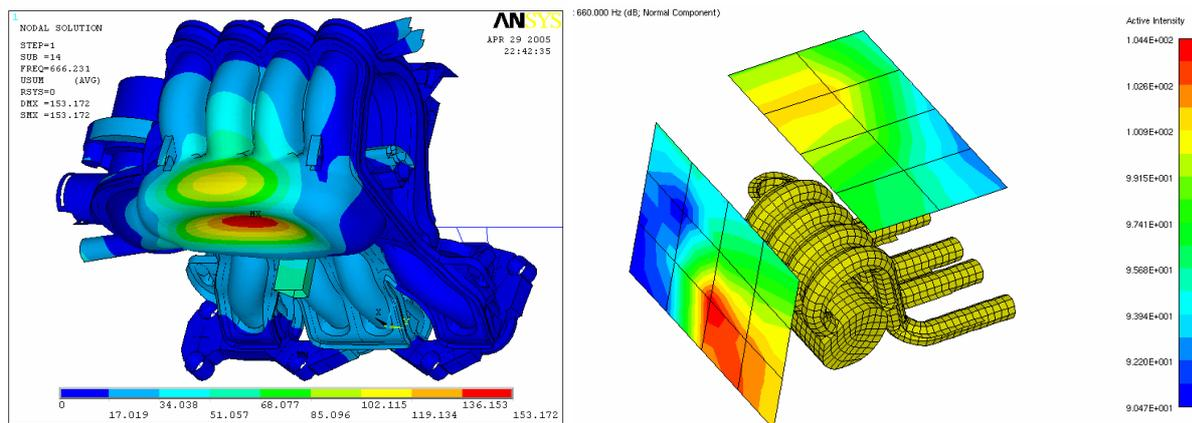
Figure 9: Detection of a particular shell-noise source. Evident structural mode of the plenum at 666.2 Hz, on the left; active intensity map [dB] on the field points mesh at 660 Hz, after the coupled FEM - IBEM analysis for the 1200 camshaft rpm case.
