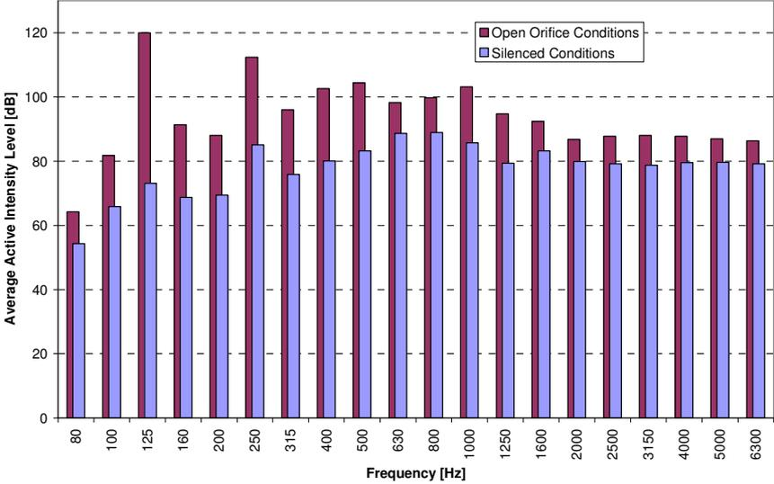
Figure 6: Effect of silenced orifice on the average sound intensity level recorded on a planar surface above the AIM, at 2000 camshaft rpm (using a 12 mm microphone spacer).
