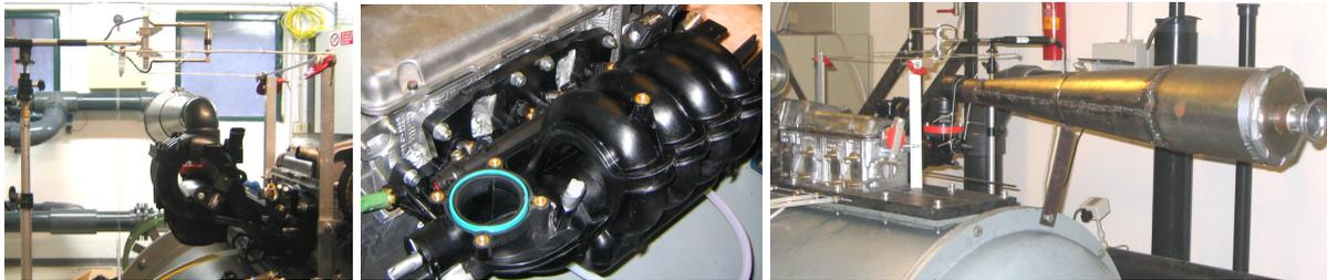
Figure 5: On the left, example of intensity probe location; on the middle, open inlet orifice condition; on the right, silenced inlet condition.
