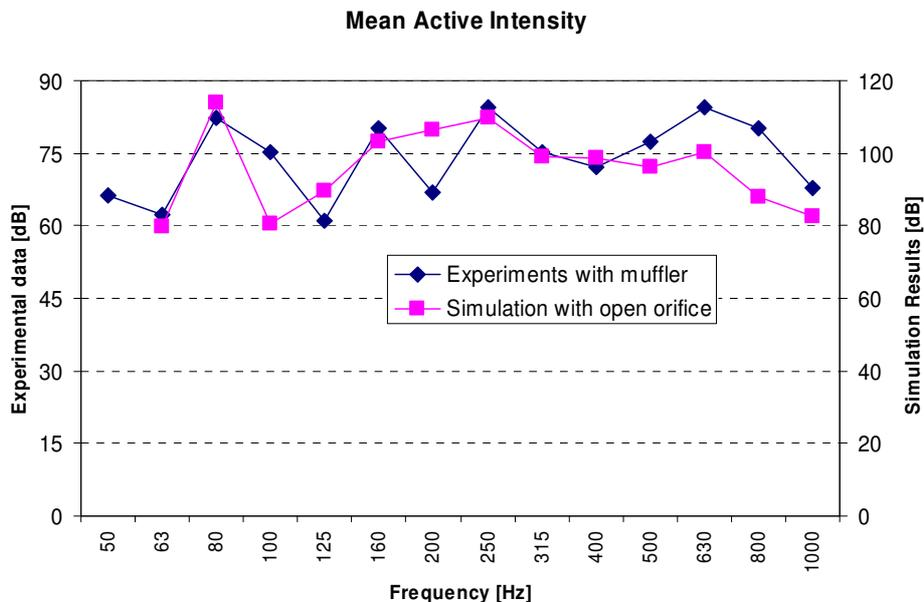
Figure 8: Average sound intensity level recorded and calculated on the two planar surfaces defined around the AIM (see Figure 2, right), at 1200 camshaft rpm (measurement performed with a 50 mm microphone spacer).
