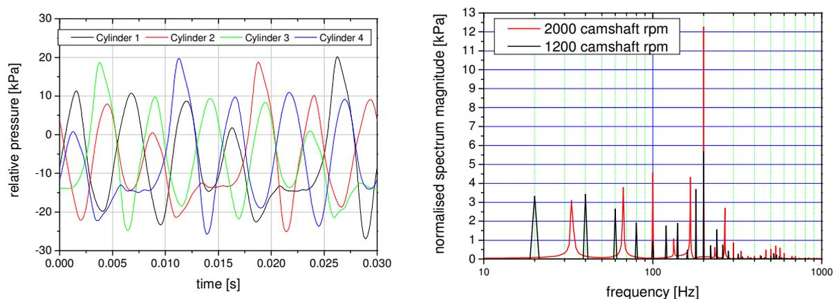
Figure 3: On the left, an example of measured pressure at the AIM's outlets (2000 rpm of the camshaft); on the right, examples of normalized pressure spectra (at 1200 rpm and 2000 rpm of the camshaft).
