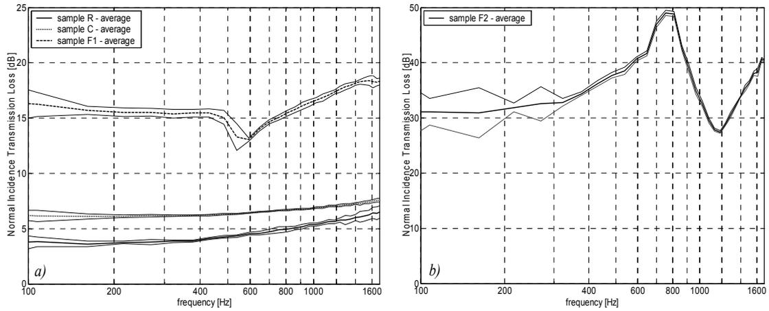
Figure 5 – Average TL data (two-load method with open-end and hard terminations) and 95%-confidence limits (thinner lines). a) sample R, C, and F1; b) sample F2.
