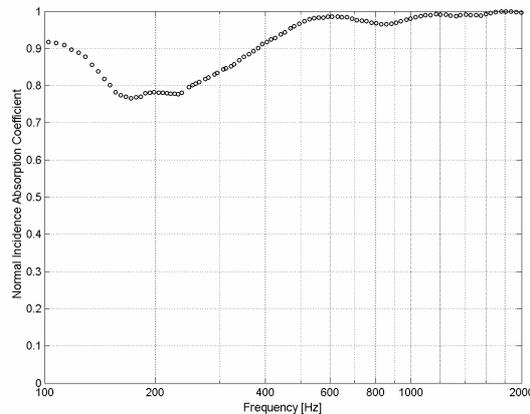
Figure 2 - Normal incidence absorption coefficient (with no backing) of the dissipative termination used in the experiment.
