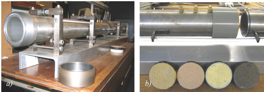
Figure 3 - Experimental setup used for the measurements: a) view of the standing wave tube from the downstream section side, b) the four tested samples and the tube sample holder.
