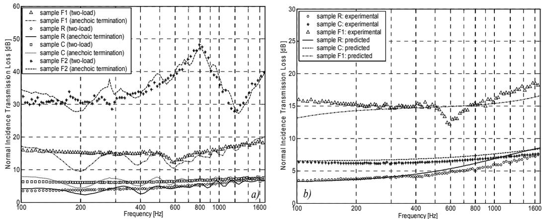
Figure 4 – a) Transmission loss measurements with the anechoic termination and the two-load method (open-end and hard terminations); b) Comparison between predicted and measured (two-load method) values of Transmission Loss for samples R, C and F1.
