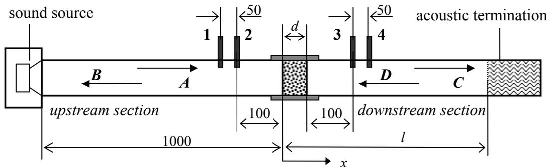
*Figure 1 – Standing wave tube geometry for the plane wave decomposition procedure.
