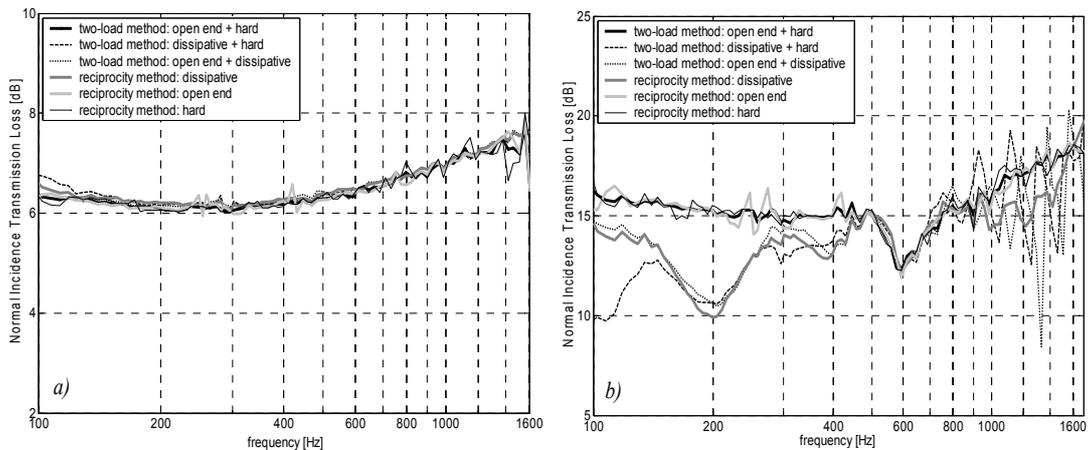
Figure 6 – The transmission loss measurements with the two-load method and the reciprocity method with different terminations. a) sample C; b) sample F1.
