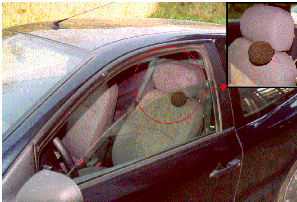
Figure 1: measurement microphone position
